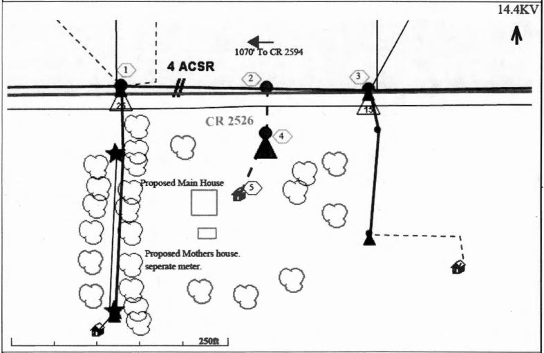
Misc. Remarks: Need to set new pole inline to single phase line then set new pole across road for temp meter pole to build house. Cost. Gave one easement need to send construction release. Need county road permit. R1/R1. MS
